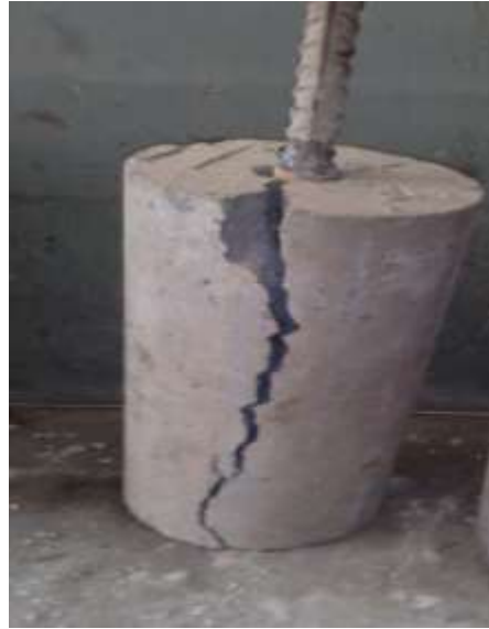
Plate (4) Splitting failure
