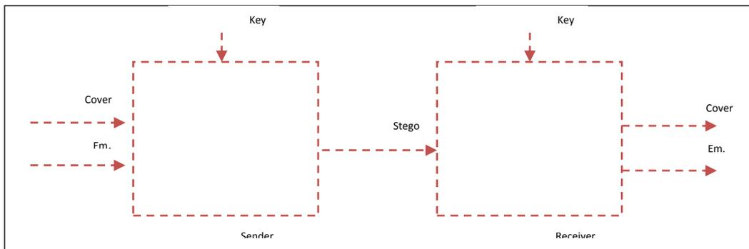
**Fig.1 Graphical Version of the Steganography System**
