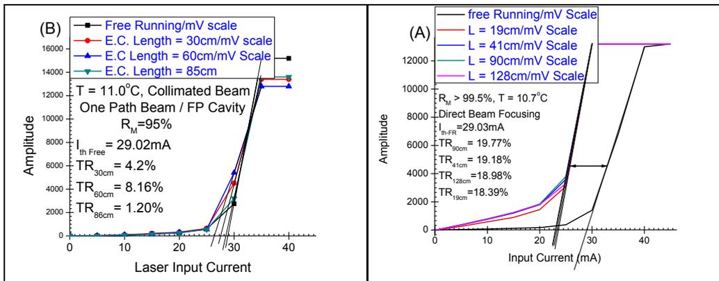
Fig.9: Threshold reduction for different (EC) lengths, A: focused and B: collimated beam geometry.
