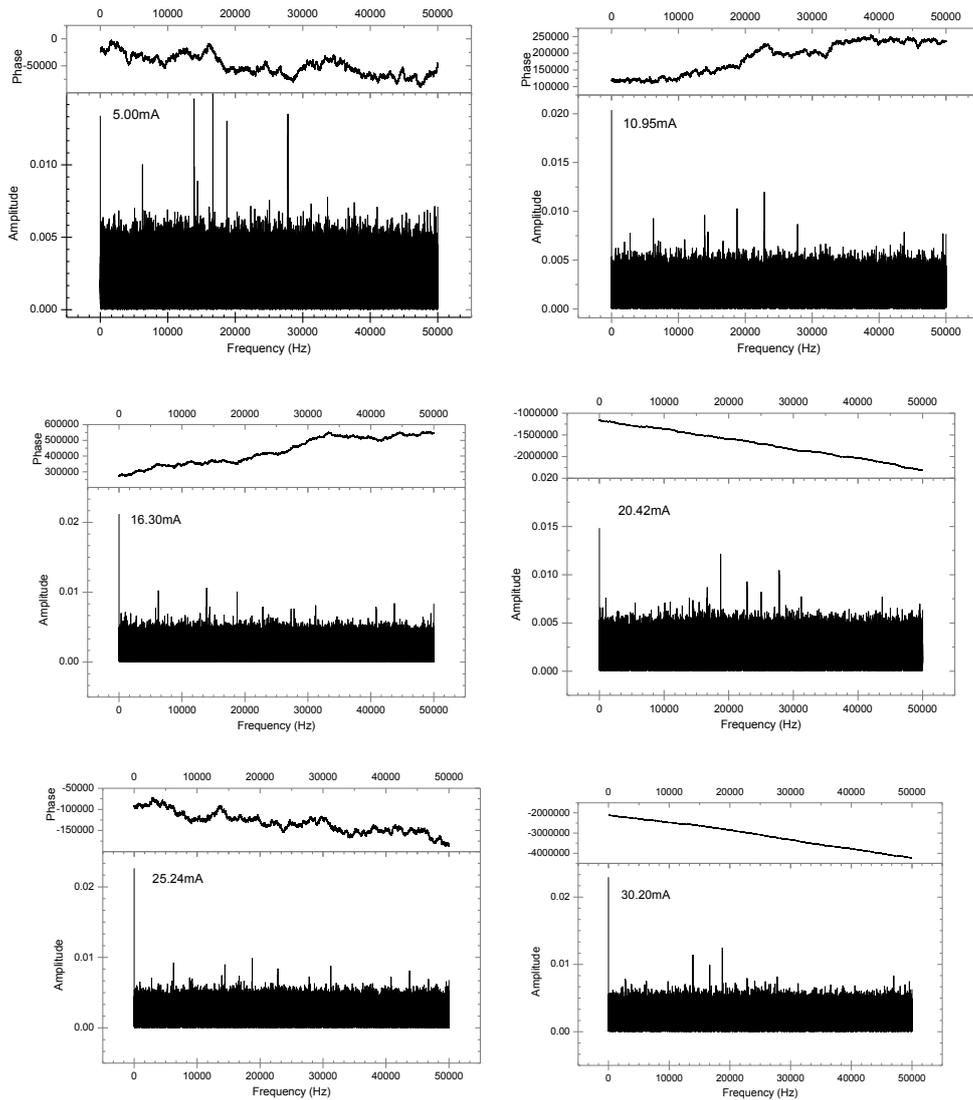
Fig. 6: Free running (FFTs) power spectra map for (DFB) Laser
