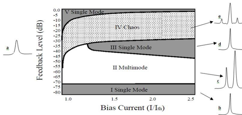
Fig. 1: Optical spectra for: a. laser without feedback. b. Regime I, c. II, d: III, and e. regime IV, according to feedback strength [9].
