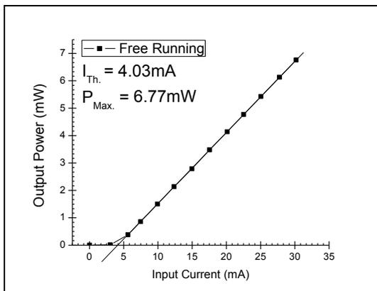
Fig.4: Solitary laser (**L/I**) curve at  $14.5C^{\circ}$ .
