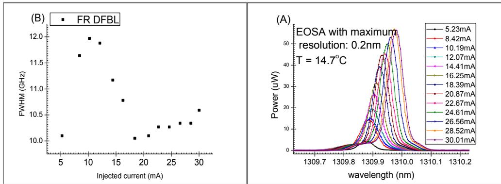
Fig. 5: Free running laser optical spectra
