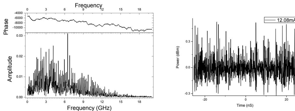
Fig. 11: Laser dynamics, time series and its power spectrum with 85cm single EC.
