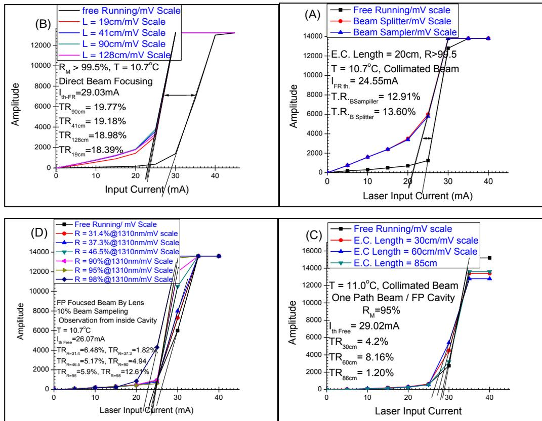
Fig.8: Threshold reduction possibilities: A: (NBS) and beam sampler, B: direct focused beam, C: collimated beam, and D: focused beam by a lens.
