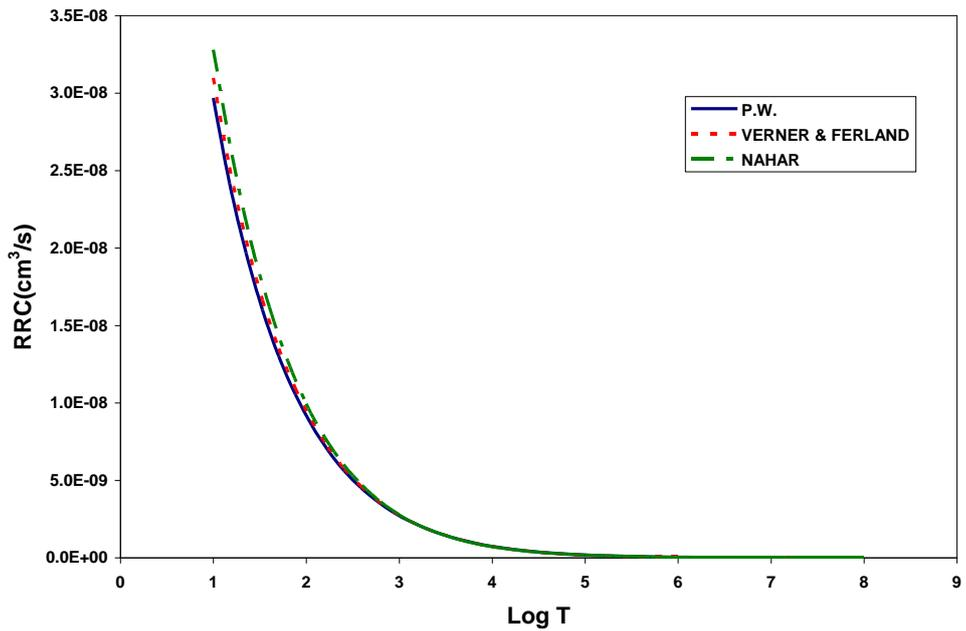
FIG.(17):Radiative recombination rate coefficient for Ni XXVII-ion compared with VERNER & FERLAND (1996) and NAHAR (2005) calculations.
