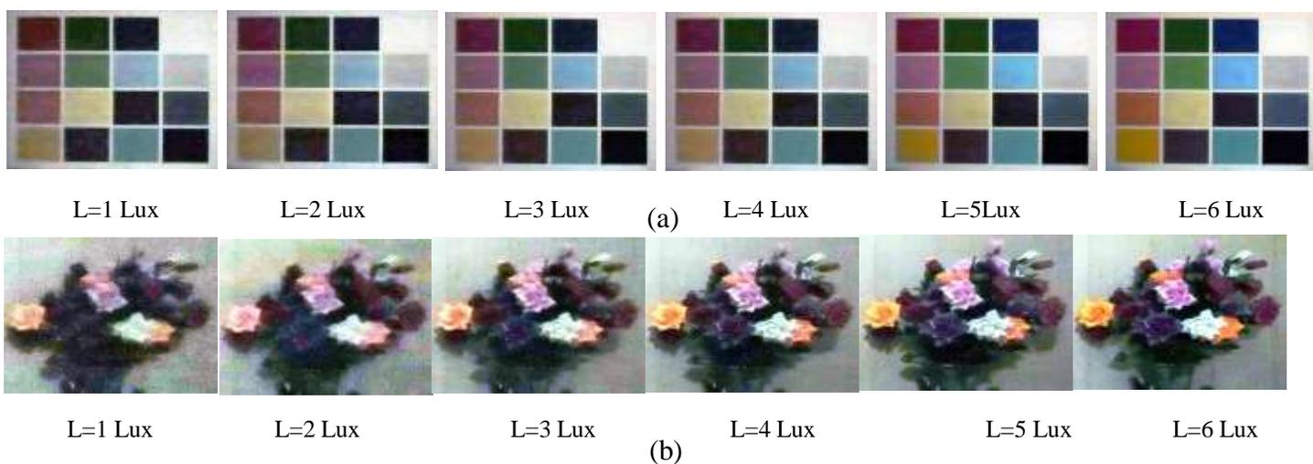
**Figure (4): The enhanced images by H.E. algorithm for captured images by SM-Cam under low lightness values. (a) Test color chart enhancement image, (b) Flowers enhanced Images**
