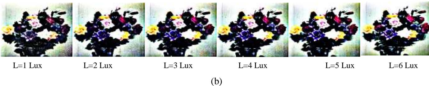
*Figure (8): The enhanced images by (W.R) algorithm for captured images by SM-Cam under low lightness values. (a) Test color chart enhancement image, (b) Flowers enhanced Images*
