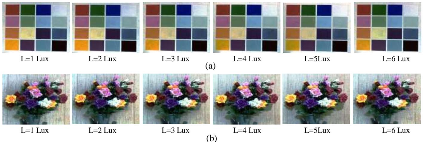
**Figure (5): The enhanced images by H.E. Algorithm for captured images by SN-Cam under low lightness values. (a) Test color chart enhancement image, (b) Flowers enhanced Images**
