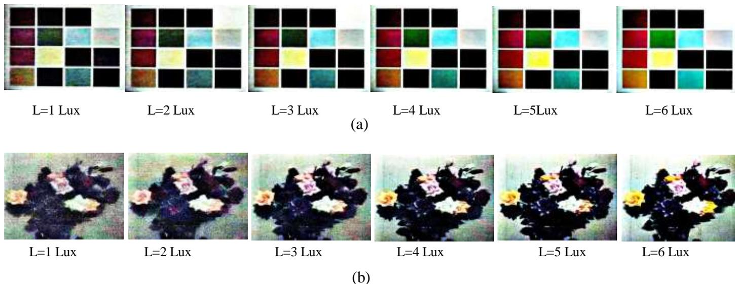
**Figure (6): The enhanced images by Retinex (R) algorithm for captured images by SM-Cam under low lightness values.(a) Test color chart enhancement image,(b) Flowers enhanced Images**
