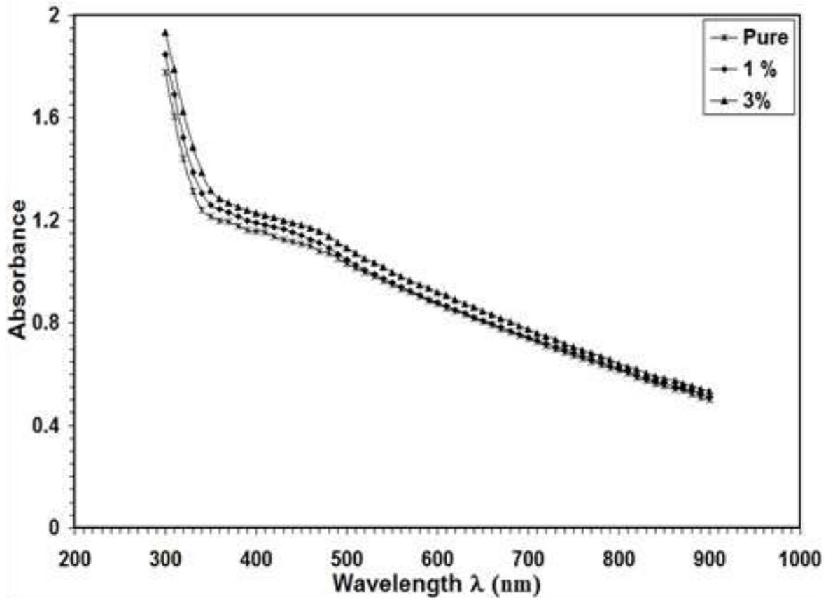
**Fig.1: Absorbance with wavelength for Fe<sub>2</sub>O<sub>3</sub> thin films and different doping of Sb concentration.**
