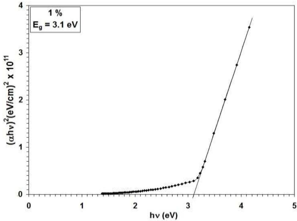
**Fig.4:  $(\alpha h\nu)^2$  against photon energy of  $\text{Fe}_2\text{O}_3$ :1%Sb concentration.**
