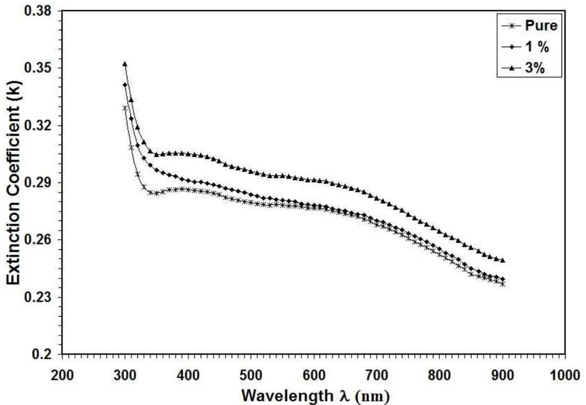
**Fig.6:  $k$  for  $\text{Fe}_2\text{O}_3$  with different doping concentration of Sb: $\text{Fe}_2\text{O}_3$  thin films versus wavelength.**
