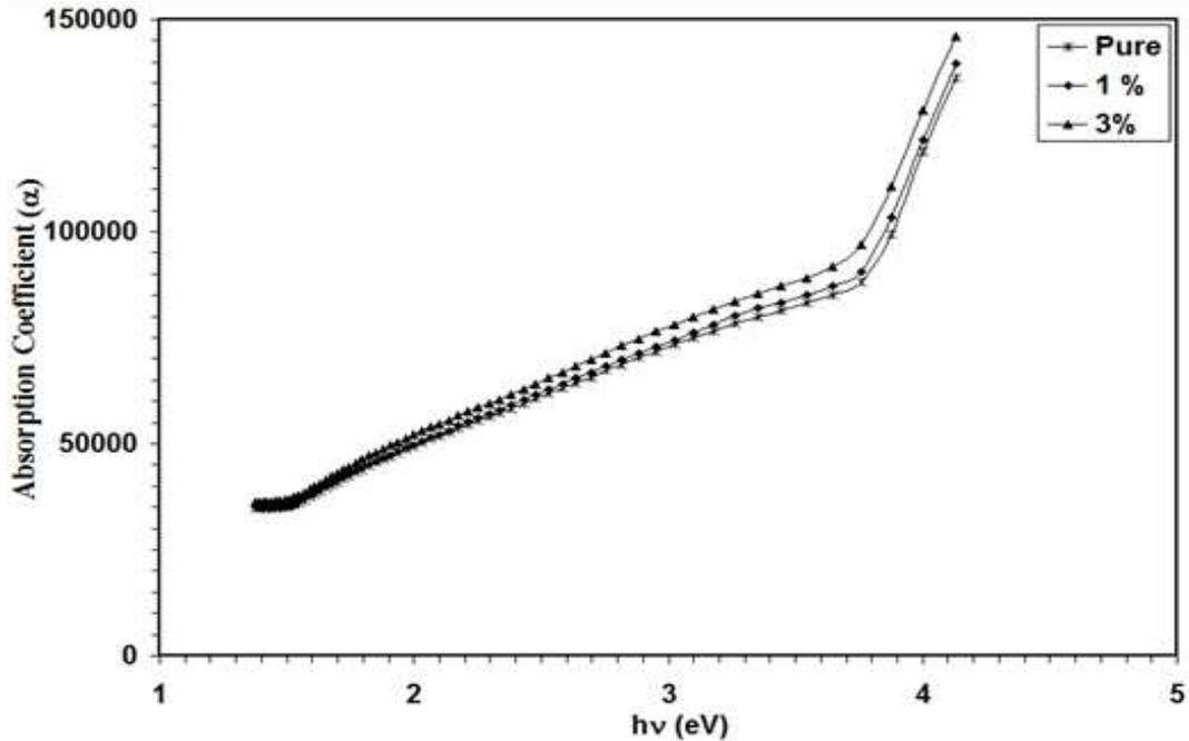
**Fig. 2:  $\alpha$  against wavelength for  $\text{Fe}_2\text{O}_3$  thin films and different doping of Sb concentration.**
