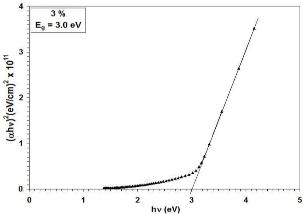
**Fig.5:  $(\alpha h\nu)^2$  against photon energy of  $\text{Fe}_2\text{O}_3$ :3%Sb concentration.**
