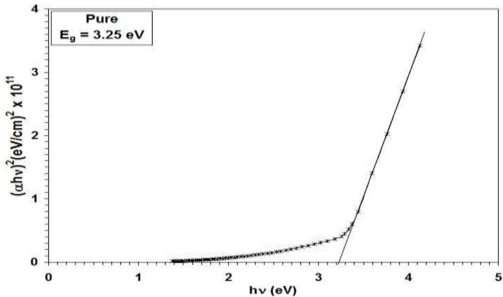
**Fig.3:  $(\alpha h\nu)^2$  against photon energy for  $\text{Fe}_2\text{O}_3$  thin films.**
