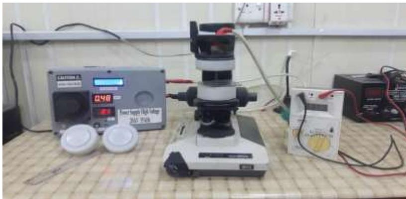
Figure (2): The locally designed DBD Plasma system.
