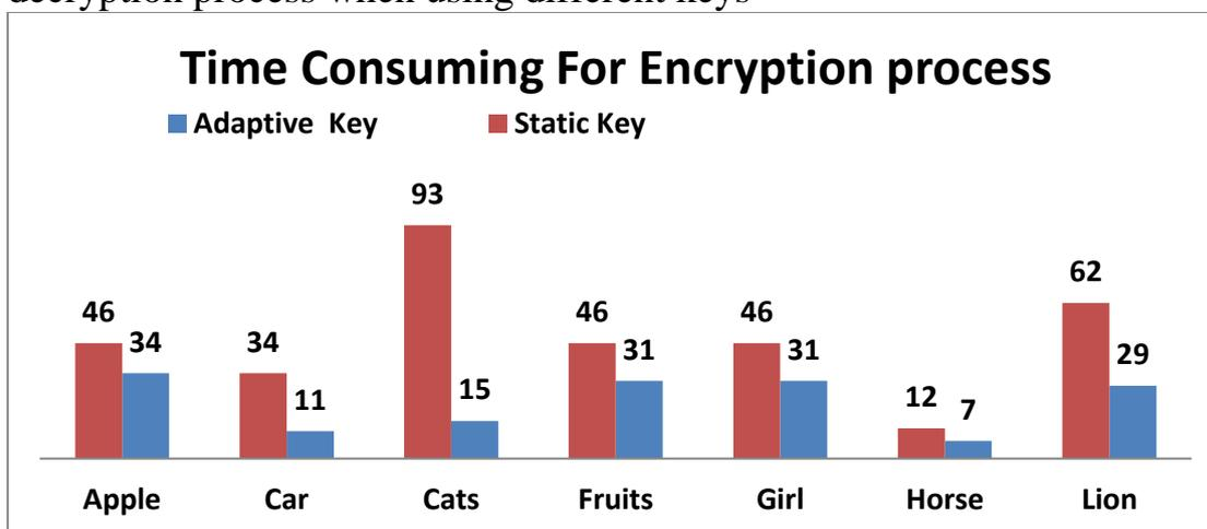
**Fig.(7) encryption time consuming for static and proposed adaptive keys**
