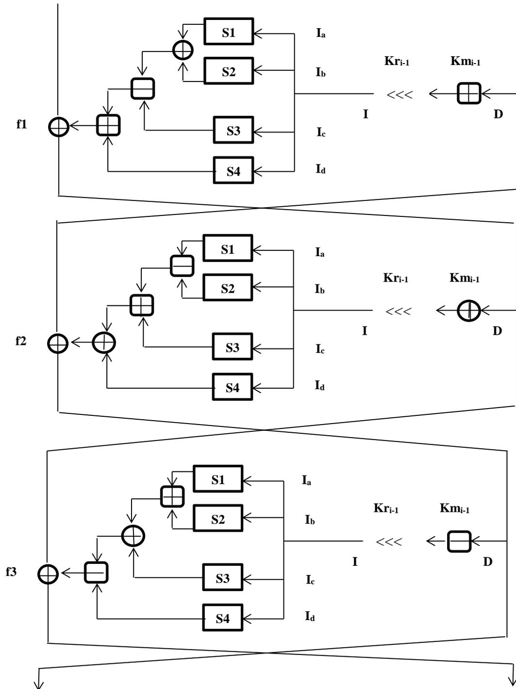
**Fig. (2) : Encryption Procedure for CAST-128 [9]**
