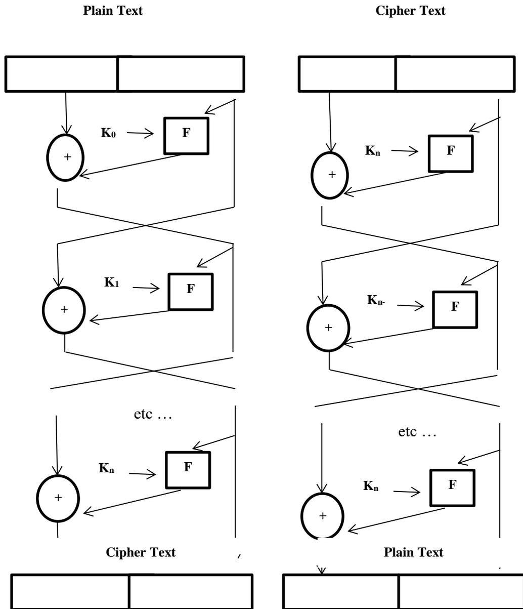
**Fig.(1) : Encryption and Decryption of CAST-128 [8].**
