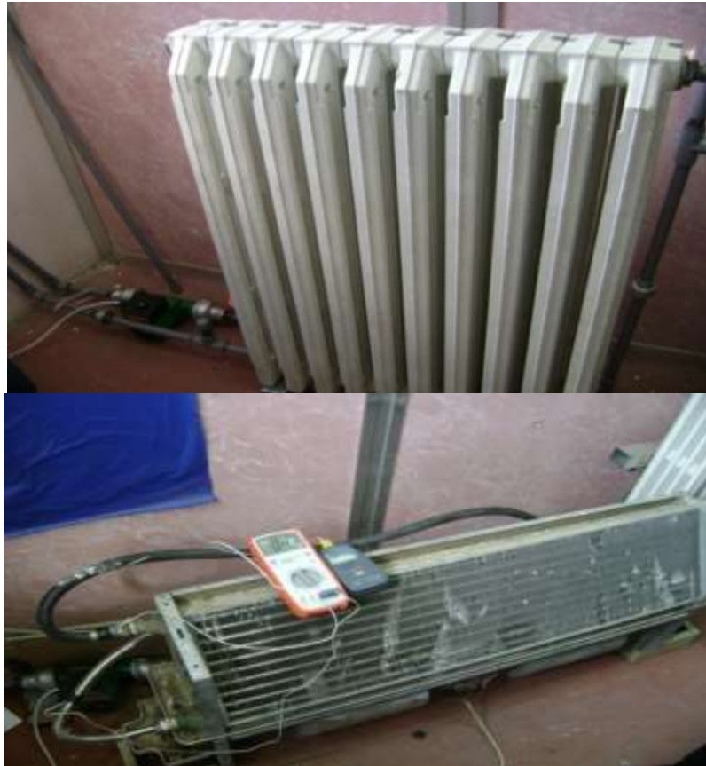
Figure (5): the iron material (a), and the Aluminum material (b) radiator types
