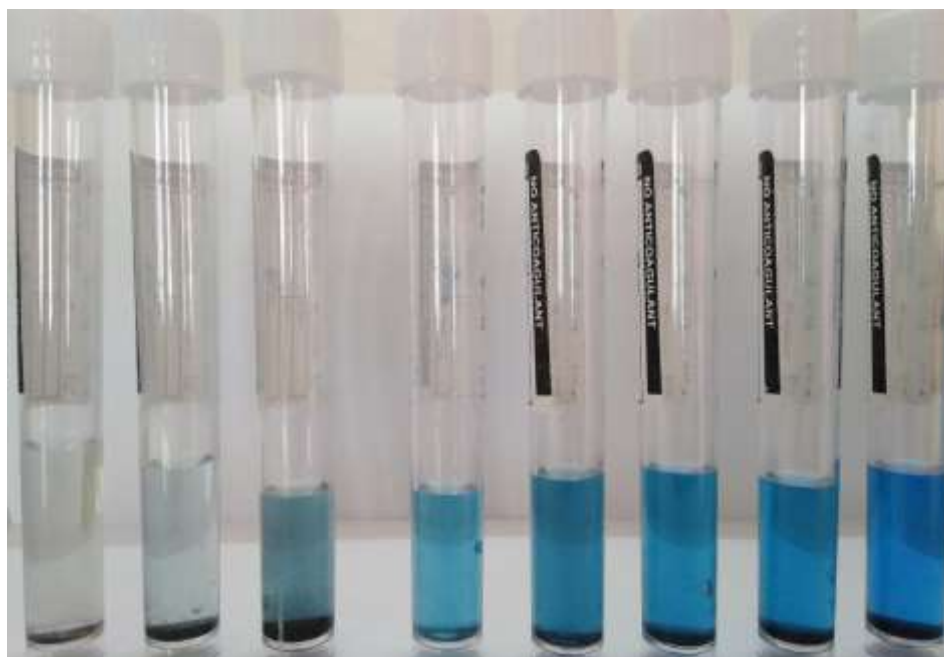
Fig.(5) Color of methylene blue (MB)/CuO nano-rice structures within 70 min of natural sunlight irradiation.
