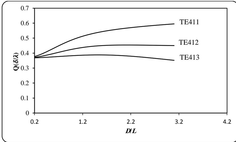
Fig.(3-d) ( $Q(\delta/\lambda)$ ) versus ( $D/L$ ) for the TE<sub>411</sub>,TE<sub>412</sub>,TE<sub>413</sub>
