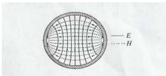
Fig.1: Field configuration for the TE<sub>11</sub> (dominant) mode in a circular waveguide.
