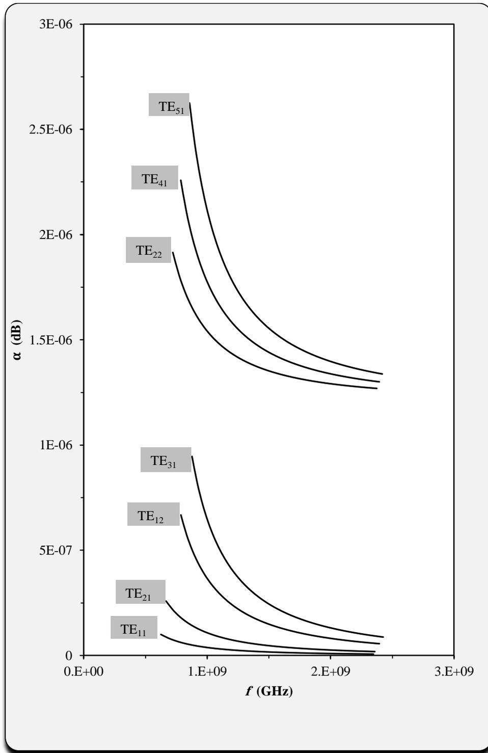
Fig.4: The attenuation constant of several higher order modes in circular waveguide.
