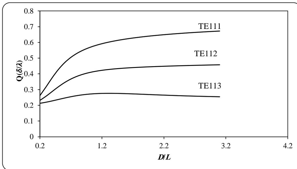
Fig.(3-a):  $Q(\delta/\lambda)$  versus ( $D/L$ ) for the TE<sub>111</sub>,TE<sub>112</sub>,TE<sub>113</sub>.
