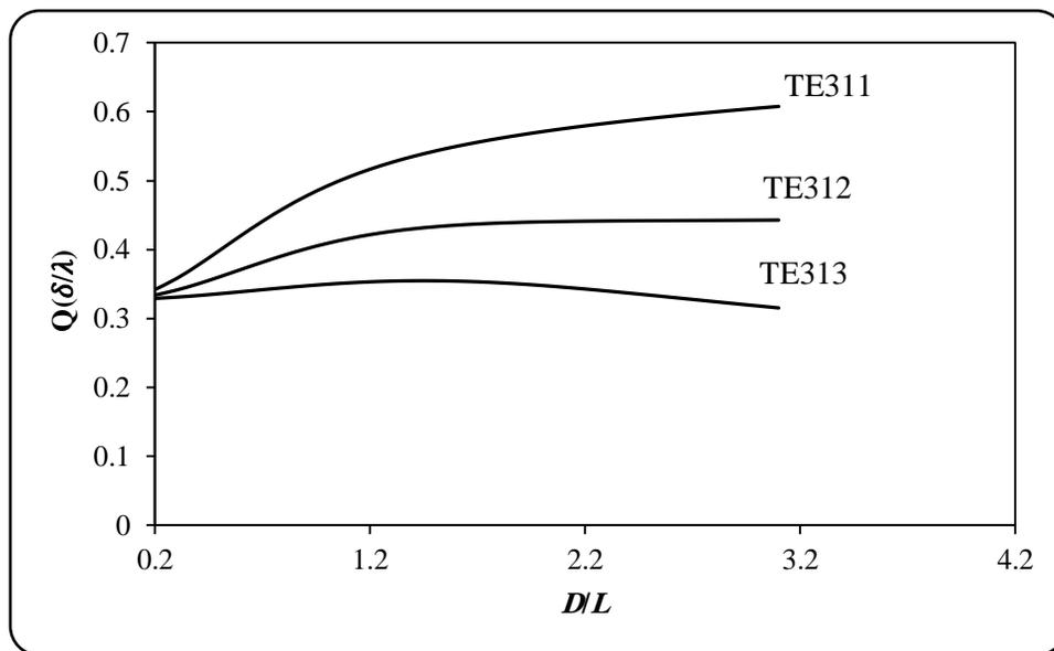
Fig.(3-c):  $Q(\delta/\lambda)$  versus  $(D/L)$  for the TE<sub>311</sub>, TE<sub>312</sub>, TE<sub>313</sub>.
