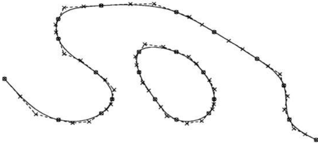
Figure 6. Bezier control focuses (crosses and ran line) decided for a standard parametric spline bend decided for the surrounded bunches.
